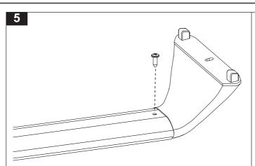
From the underside of the cross bar insert the phillips head screw.
