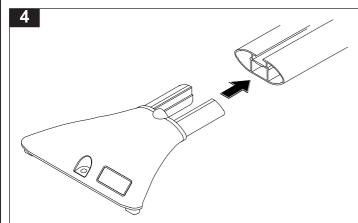
Insert the Sportz leg fully into the cross bars, a rubber mallet may be required to knock the leg in place.
