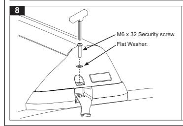
Place the flat washer over the M6 Security screw and then fasten to the stainless steel strap. **TIGHTEN TO 3-4N/m. DO NOT OVER TIGHTEN.**
