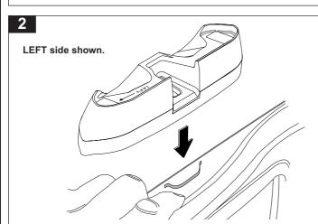
Place the correct roof pad on the roof up against the edge of the roof channel. The pads are marked LEFT and RIGHT with the ARROW facing towards the front of the vehicle once installed.
