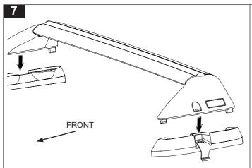
Place the assembled cross bars onto the front and rear roof pads.
