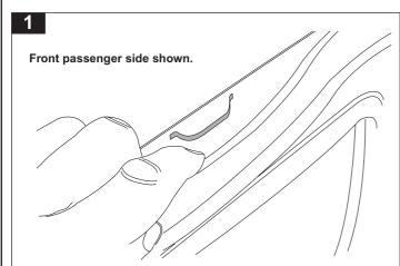
Locate the Front and Rear metal lugs in the roof gutter. The **Front Lug is 340mm** from the back edge of the winscreen rubber, the **Rear Lug is 1010mm** from the back edge of the winscreen rubber. Open doors and gently lift and peel the rubber strip back to expose the lugs at these points.
