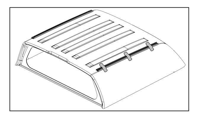
Now place the track onto the canopy. Once in position (pg1), using masking tape, apply 3 strips at the front, middle and the rear of the track as shown. This allows the track to be held in position. Using a sharp  $\emptyset$ 6.5mm drill bit, hold the drill perpendicular to the surface of the canopy, apply minimal pressure and proceed to drill. Make sure both the inner and outer skins are drilled through. Remove any swarf with a vacuum.
