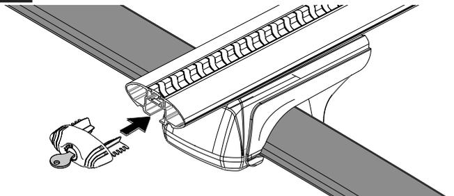
Insert Locking End Cap and remove key
