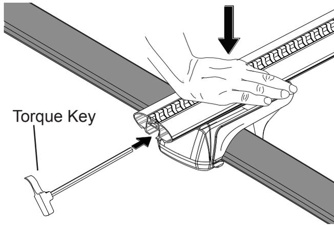
Fasten each leg alternately using the supplied Torque allen key.
