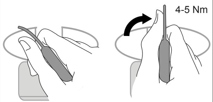
With Torque Key inserted, turn clockwise until handle straightens out as shown above. This indicates 4-5 Nm. More pressure may be required in extreme climates.
