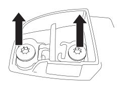
A T40 Torx key is required to remove the screws.
