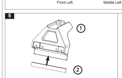
If not already attached, attach a rubber boot (item 2) to the base of each leg.
