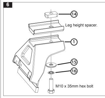
When using 3 Crossbars, leg height spacers are required for the Front & Rear crossbar to get all three level.
