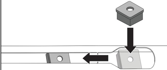
**2** Install the Legs into the Foam Special Nuts as shown. Tighten with Torque Allen Key provided.
