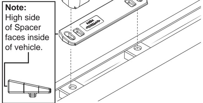
**3** The Crossbars should be spaced between 700mm and 800mm apart.
