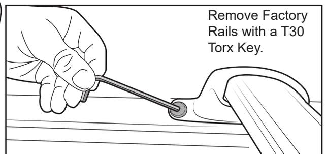
Remove Factory Rails with a T30 Torx Key.
