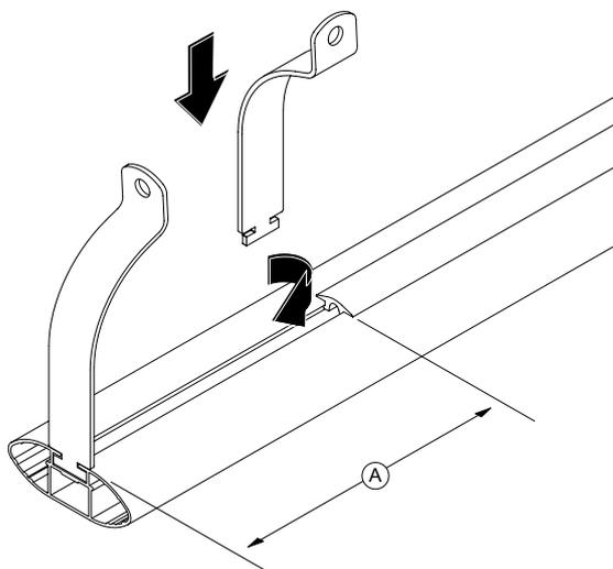
Cut the rubber buffer strip as shown, (B) = 110mm (for 4" conduit) and 160mm (for 6" conduit). Angle the pipe clamps back to allow room for the conduit. Place the rubber strip in between the clamps. Repeat steps 1 & 2 for the second set of clamps. Make sure the clamps are parallel to each other.
