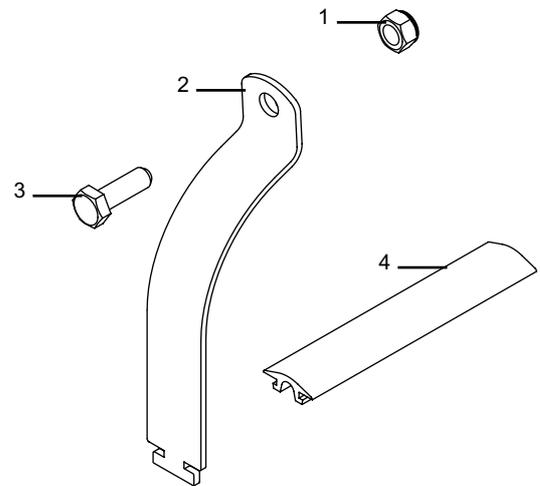
Trim the rubber buffer strip as shown, (A) = 120mm (for 4" conduit) and 170mm (for 6" conduit). Insert the Sportz pipe clamps vertically into the Sportz bar channel. Once inserted rotate 90° as shown.
