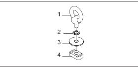
Assemble the shake proof washer and flat washer onto the eyebolt (shake proof washer first). Screw the channel nut onto the eyebolt with the grooves facing the eye bolt.
