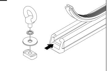
Position the eyebolt and locate the channel nut into the crossbar recess, turn the attachment bolt so that the channel nut rotates and locates across the crossbar. Trim rubber buffer strip to suit.
