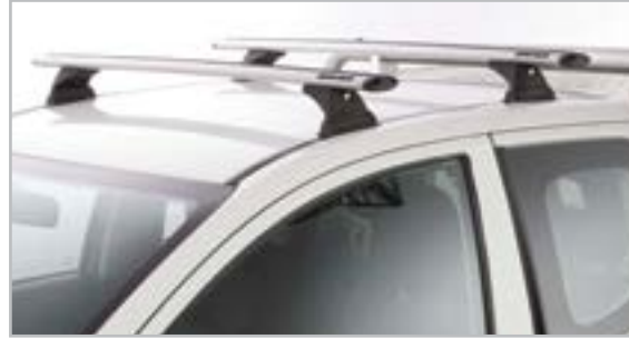
4.2 RLT500 Position your roof rack system along the track
